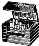
This kit of ceramic, slug-tuned coil forms meets coil requirements encountered by development labs. Amateurs and experimenters. Includes 15 coil forms (3 each of 5 different types), 19 powdered iron slugs, 5 silver-plated brass slugs, and complete set of mounting hardware. Coils covering 50 kc to 200 mc can be wound with the coil forms and slugs supplied. Diameter of forms range from 3/16" to 1/4"; mounted heights from 1/16" to 1/8". Shpg. wt., 13 oz.
