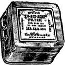
Feed-through, high-pass type interference filters for use at antenna terminals of TV receiver. Attenuate interference from 0 to 50 mc as much as 60 db. Effectively reduces signal from diathermy, radio stations, industrial equipment, etc. TV-72 for 72-ohm lines. TV-300 for 300-ohm lines. \*For sets with 20 mc IF's. †For 20 and 44 mc IF's. Metal case 2x2x1½". Shpg. wt., ½ lb.
