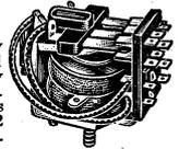
High-quality, general purpose relay. Particularly useful for transmitters, power supply control and remote switching applications. Have heavy-duty contacts rated at 4 amps. AC coils for 50-60 cycles. Moisture resistant against humidity. Withstands shock encountered in mobile applications. #6-32 mounting stud. Size, 1 1/2" x 1 1/2" x 1 1/2". Shpg. wt., 8 oz.
