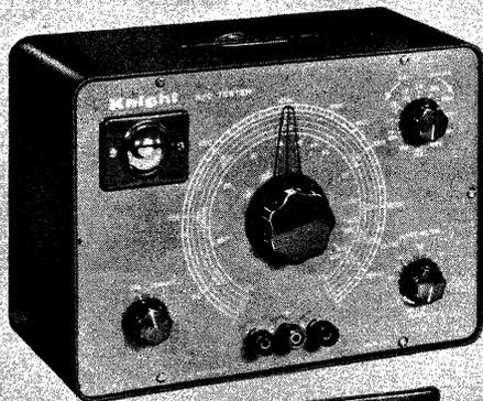
Excellent for lab and service shop. Accurately analyzes capacitors and resistors.
