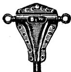
Provides weatherproof, strong cable connections to half-wave doublet antennas and also serves as center insulator. Watertight aluminum housing. Antenna elements connect to forged steel eye-bolts. Internal soldering connections for coax cable. Rubber sleeve for small diameter cable. Includes cement, eye-bolts rubber sleeve, screws, 2 housing sections, and instructions. Shpg. wt., 1 lb.
