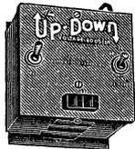
**Type LB2 (N).** Same as type LB2 described above, but has neon indicator which operates when output voltage is too high—indicates when regulator should be turned off. Indicator light goes on when output voltage of regulator reaches 126 volts. Simplifies operation. **63 G 987. List, \$11.95. NET.....7.03**
