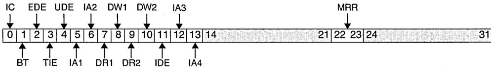
**Figure 25-15. Debug Status Register (DBSR)**
