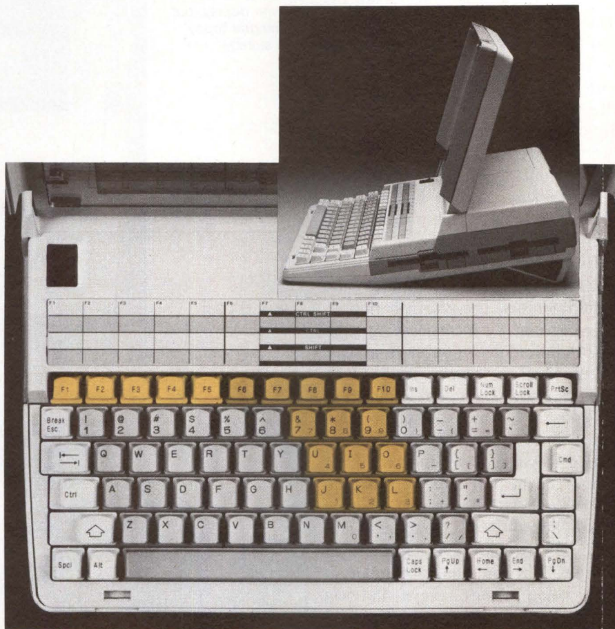
The keyboard on the Data General/One (inset) is not identical to the IBM PC's, because the function keys are parallel to the screen rather than clustered on the left side of the keyboard. Also, the numeric keypad, which is on the right side of the IBM PC's keyboard, is incorporated in the character keys on the Data General model.
