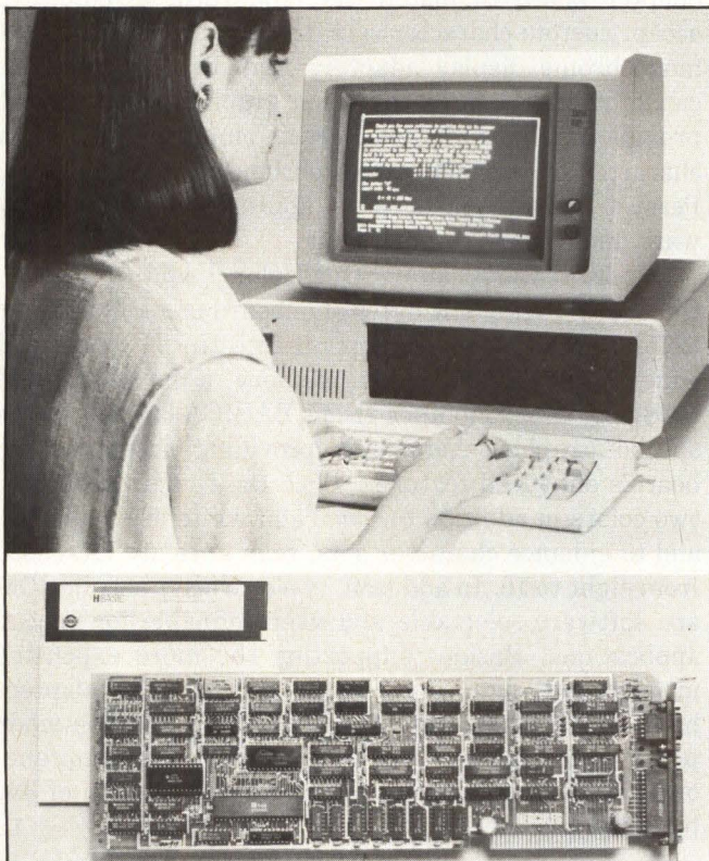
The Hercules graphic card displays up to 90 characters per line and 43 lines per screen on a monochrome monitor, in an enhanced, condensed-display mode.
