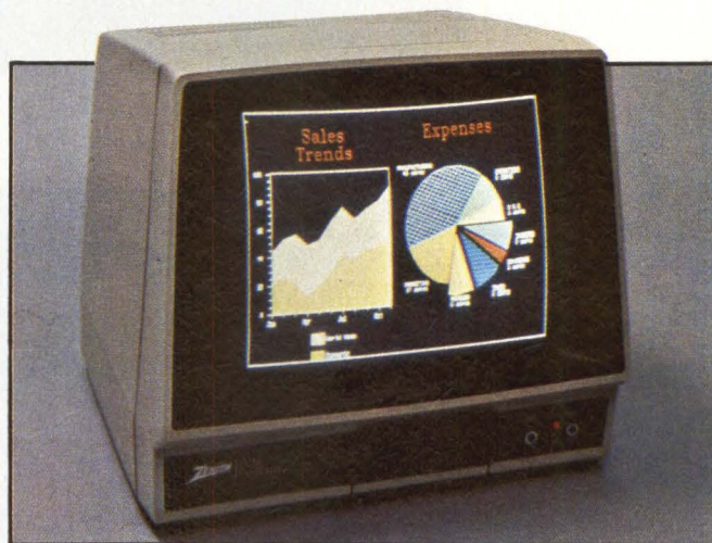
Matching the IBM PC, Zenith Data Systems' Z-150 comes with built-in monochrome and color capability, and can dynamically switch from 320-by-400 to 640-by-425-dot resolution depending on the application requirements.
