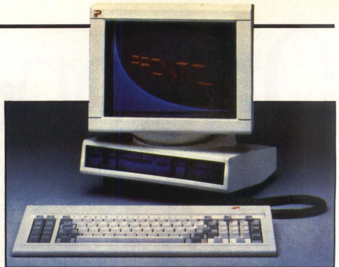
The Pronto Computer graphics adapter has three bit planes, a resolution of 640 dots by 480 dots and up to eight levels of gray scale or eight colors chosen from a 16-color palette.
