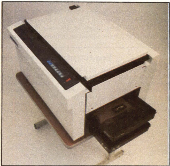
Exterior view of M3071 shows 250-sheet paper cassettes. The machine prints at 20 pages per minute with a resolution of 240 dots per inch.
