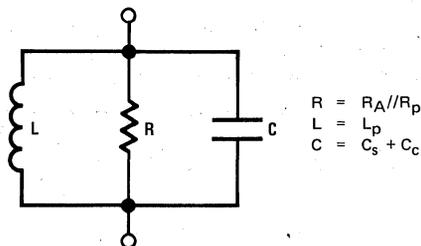
**FIGURE 4.** Simplified Inductive Source Network
