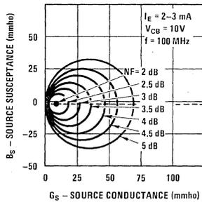
Common Base Noise Figure vs Source |Y<sub>S</sub>|
