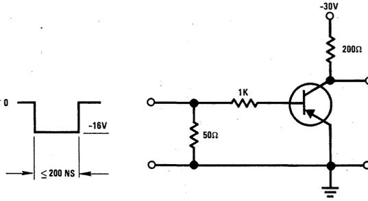
FIGURE 1. Saturated Turn On Switching Time Test Circuit
