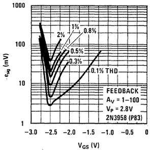
FIGURE 12. Distortion With  $V_p = 2.8V$ , With Linearization
