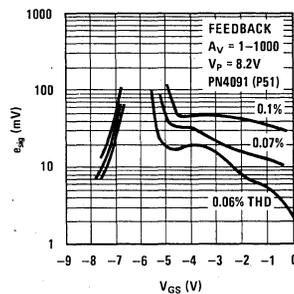
**FIGURE 16. Distortion For Circuit of Figure 14**
