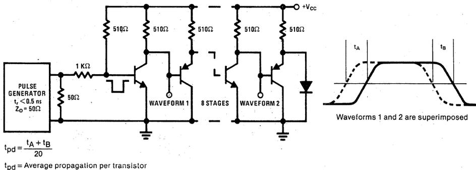
FIGURE 3. Circuit for Measurement of Propagation Delay
