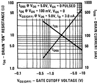
"ON" Resistance vs Drain Current
