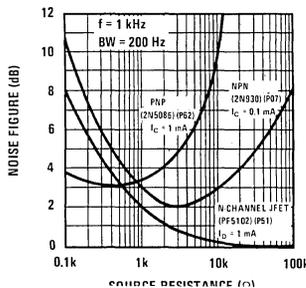
FIGURE 1. Bipolar and JFET Transistor Noise Comparison
