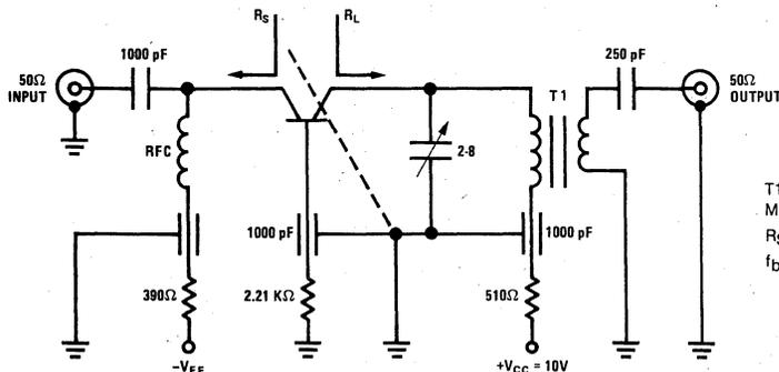
T1 - 3:1 ratio No. 22 Bifilar on Micrometals Toroid, P/N T30-12
