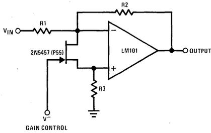
Voltage Controlled Variable Gain Amplifier
