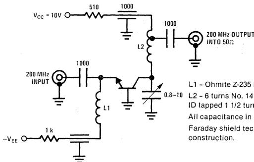
L1 - Ohmite Z-235 RF choke
