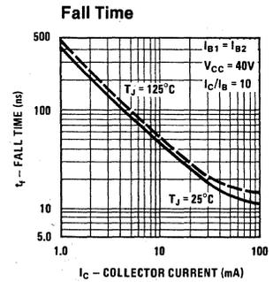
TRANSIENT CHARACTERISTICS ( $-T_J = 25^\circ\text{C} - T_J = 125^\circ\text{C}$ )
