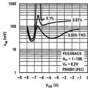
FIGURE 13. Distortion With  $V_p = 8.2V$ , With Linearization
