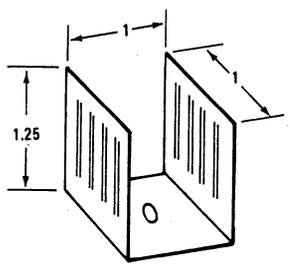
Mount transistor under heatsink and apply thermally conductive compound between contact surfaces.
