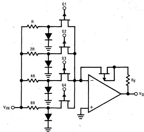
$$V_0 = -V_{IN} \frac{R_F}{R} (\bar{G}_1 2^0 + \bar{G}_2 2^{-1} + \bar{G}_3 2^{-2} + \bar{G}_4 2^{-3})$$
