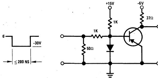
FIGURE 2. Saturated Turn Off Switching Time Test Circuit
