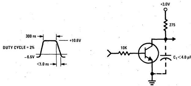
FIGURE 1. Delay and Rise Time Equivalent Test Circuit
