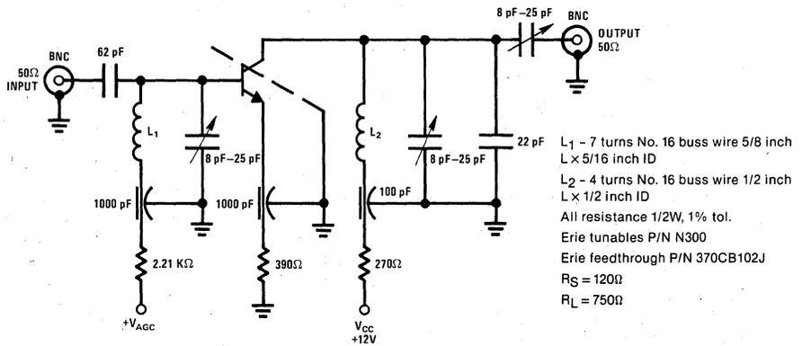
FIGURE 1. SE5055 45 MHz Gain, Noise Figure, AGC Circuit
