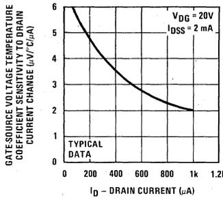
**FIGURE 3.** Gate-Source Voltage Temperature Coefficient Sensitivity to Drain Current Change vs Drain Current (Single Device)
