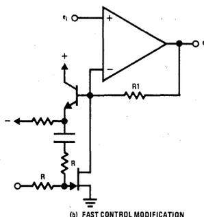
FIGURE 8. Circuit to Reduce Distortion
