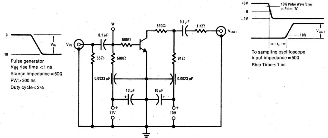
FIGURE 1. Charge Storage Time Measurement Circuit
