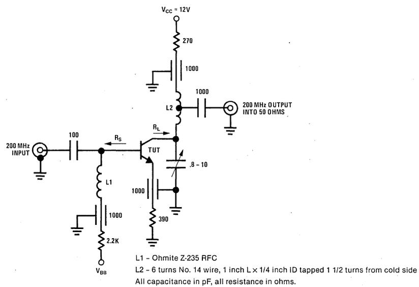
FIGURE 3. Unneutralized 200 MHz PG NF Test Circuit
