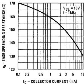
Base Spreading Resistance vs Collector Current
