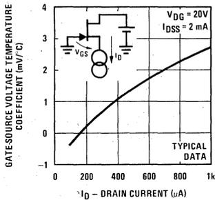
**FIGURE 2.** Gate-Source Voltage Temperature Coefficient vs Drain Current (Single Device)
