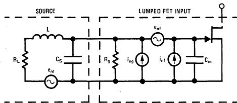
FIGURE 8. JFET Amplifier with an Inductive Source
