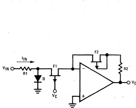
FIGURE 1. Current Mode Analog Switch
