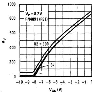
**FIGURE 15. Gain For Circuit of Figure 14**
