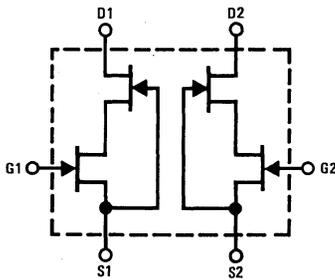
FIGURE 1a. Cascode Configuration
