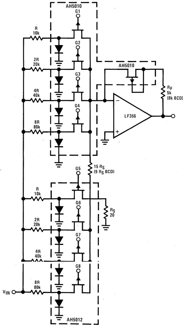
$$V_O = -V_{IN} \frac{R_F}{R} \left[ \bar{G}_1 2^0 + \bar{G}_2 2^{-1} + \bar{G}_3 2^{-2} + \bar{G}_4 2^{-3} + \frac{1}{16} (\bar{G}_5 2^0 + \bar{G}_6 2^{-1} + \bar{G}_7 2^{-2} + \bar{G}_8 2^{-3}) \right]$$
