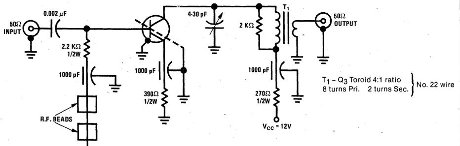
V<sub>acc</sub> FIGURE 1. 45 MHz Power Gain Circuit
