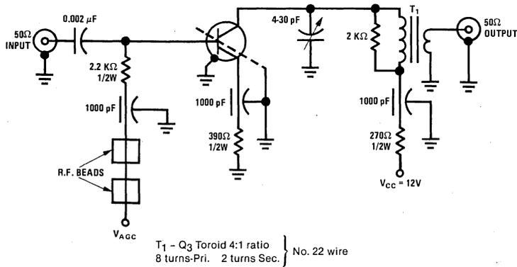
FIGURE 1. 45 MHz Power Gain Circuit
