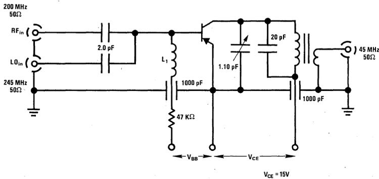
FIGURE 2. 200 MHz Conversion Gain Test Circuit
