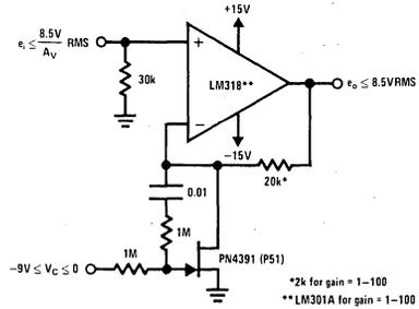
**FIGURE 14. Amplifier With Gain Range = 1–1000**
