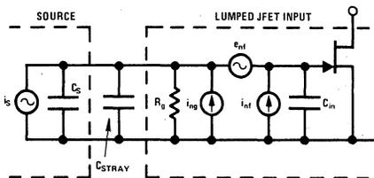
FIGURE 7. JFET Preamplifier with a Capacitive Source
