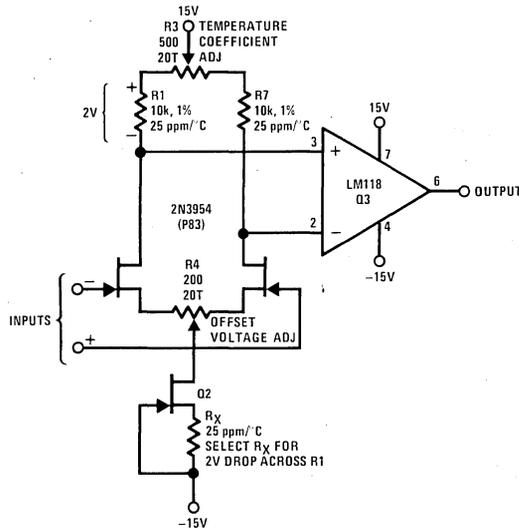
**Note 1:** The temperature coefficient can typically be adjusted (by R3 and R4) to less than  $5 \mu V/^{\circ}C$  from  $-25^{\circ}C$  to  $+85^{\circ}C$ .
