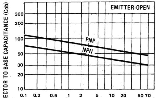
COLLECTOR TO BASE VOLTAGE ( $V_{CB}$ ) -- V
