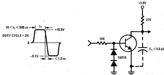
FIGURE 2. Storage and Fall Time Equivalent Test Circuit
