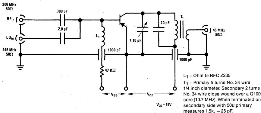
**FIGURE 2. 200 MHz Conversion Gain Test Circuit**
