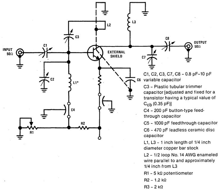
**FIGURE 1. Neutralized 450 MHz Gain and Noise Figure Circuit**
