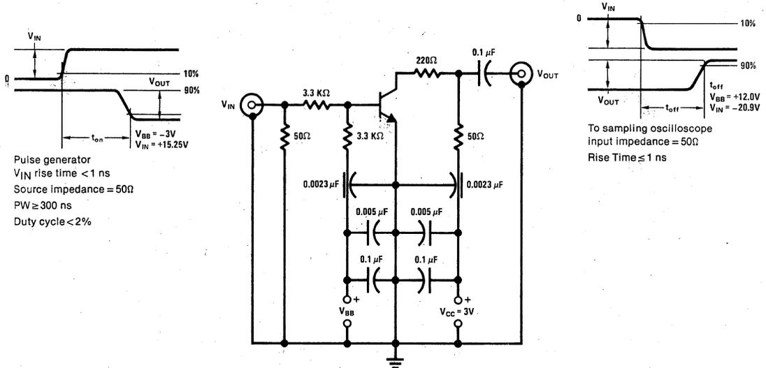
FIGURE 2.  $t_{ON}$ ,  $t_{OFF}$  Measurement Circuit
