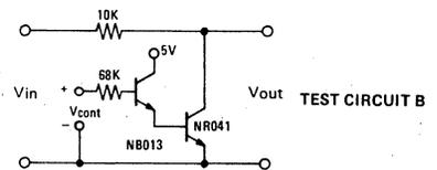
NOTE: ATTENUATION = 20 log<sub>10</sub>  $\frac{V_{out}}{V_{in}}$
