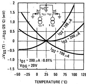
**FIGURE 5.** Differential Gate-Source Voltage vs Temperature for a Typical 2-Chip Dual JFET (10  $\mu V/^\circ C$  Unit)
