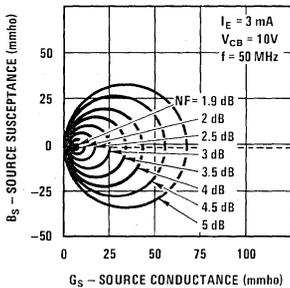
Common Base Noise Figure vs Source |Y<sub>S</sub>|
