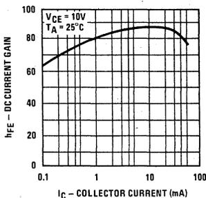
**Current Gain at 100 MHz vs Collector Current**
