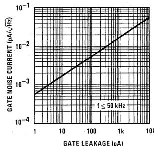
FIGURE 3. Current Noise vs. Gate Leakage Current
