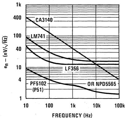
FIGURE 2. Discrete JFET and Op Amp Noise Comparison
