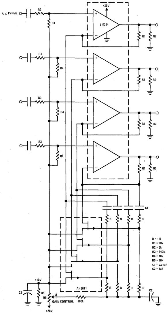
FIGURE 17. Quad Gain Control
