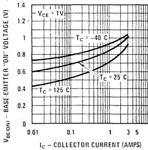
**Base-Emitter Voltage vs Collector Current**
