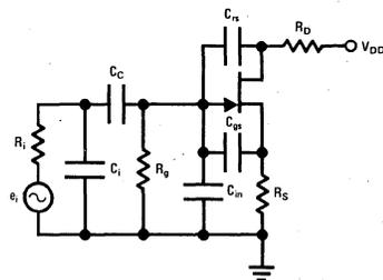
FIGURE 5. A Typical Resistive Source JFET Amplifier
