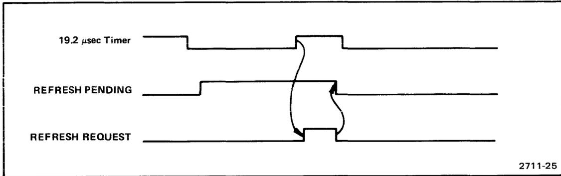
Fig. 8-2. Asynchronous Refresh Timing for High-Speed Memory.
