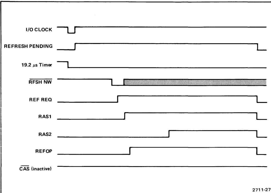
Fig. 8-4. High-Speed Memory Refresh Operation.
