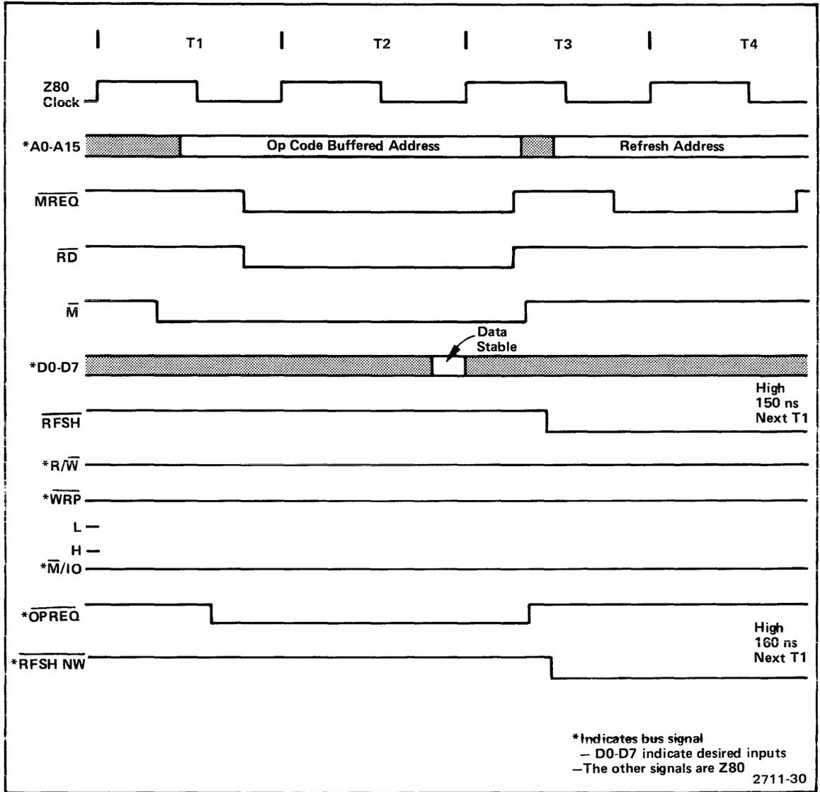
Fig. 9-1. Assembler Processor Operation Code Read Timing.
