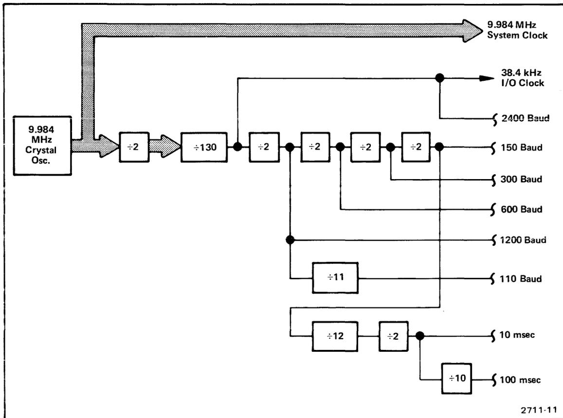
Fig. 3-2. Baud Rate Clock Divider.
