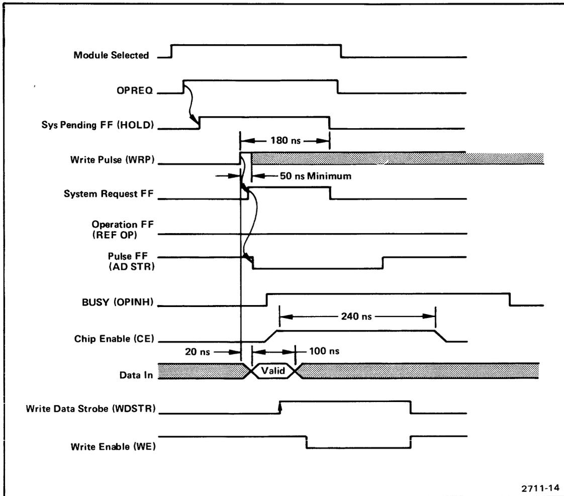
Fig. 4-3. 16K Dynamic RAM Memory Write Operation.
