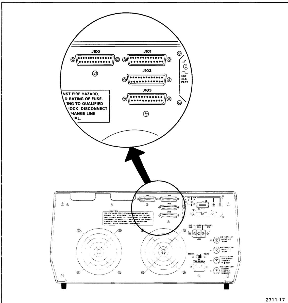
Fig. 5-3. 8001/8002A  $\mu$ Processor Lab RS-232-C I/O Ports.
